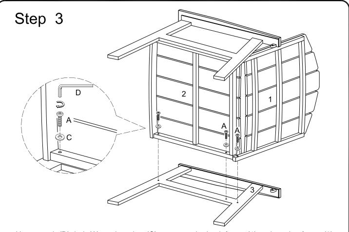
Use wrench (D), bolt (A), and washer (C) to secure the back frame (1) and seating frame (2) to the side frame (3).
